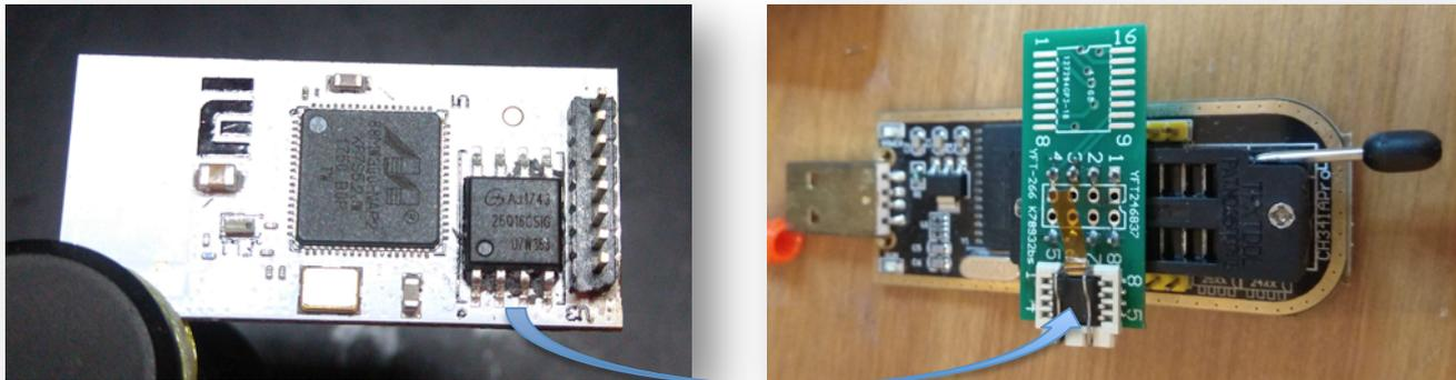
*Unsolder the SPI flash to read it directly*
